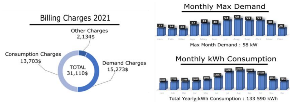
Figure A.8: System annual electricity consumption and billing charges
