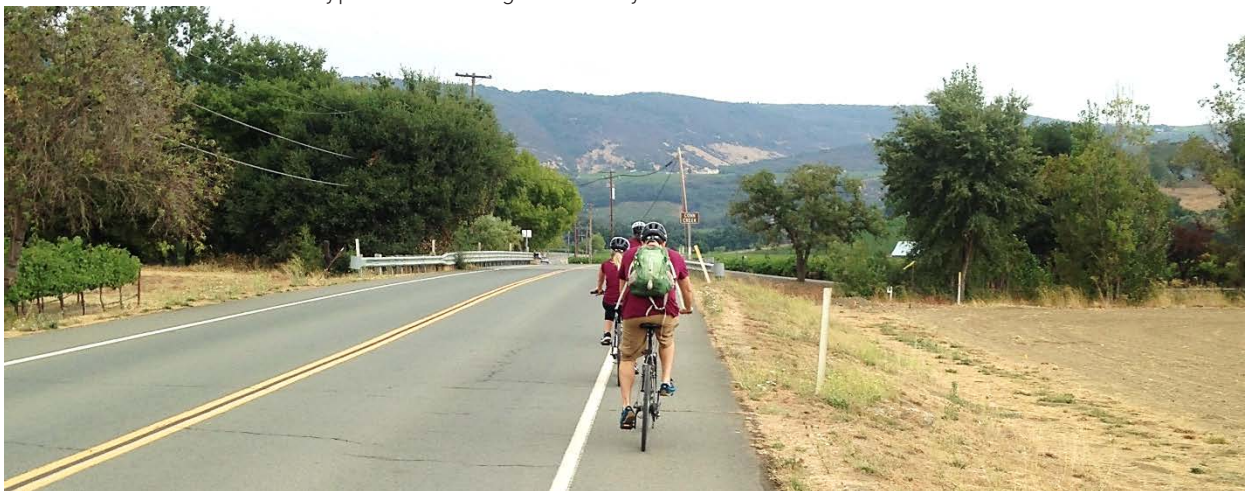
Figure 8. Relatively high Levels of Traffic Stress on a bike lane <6' on a local road in Sonoma County. Higher ADT levels and prevailing speed will negatively impact Levels of Traffic Stress.
