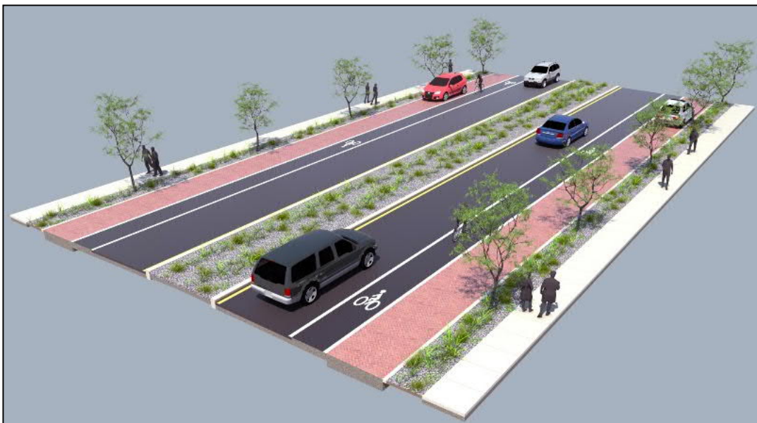
Figure 18 - Traveled Way, Bike Lane, and Shoulder
